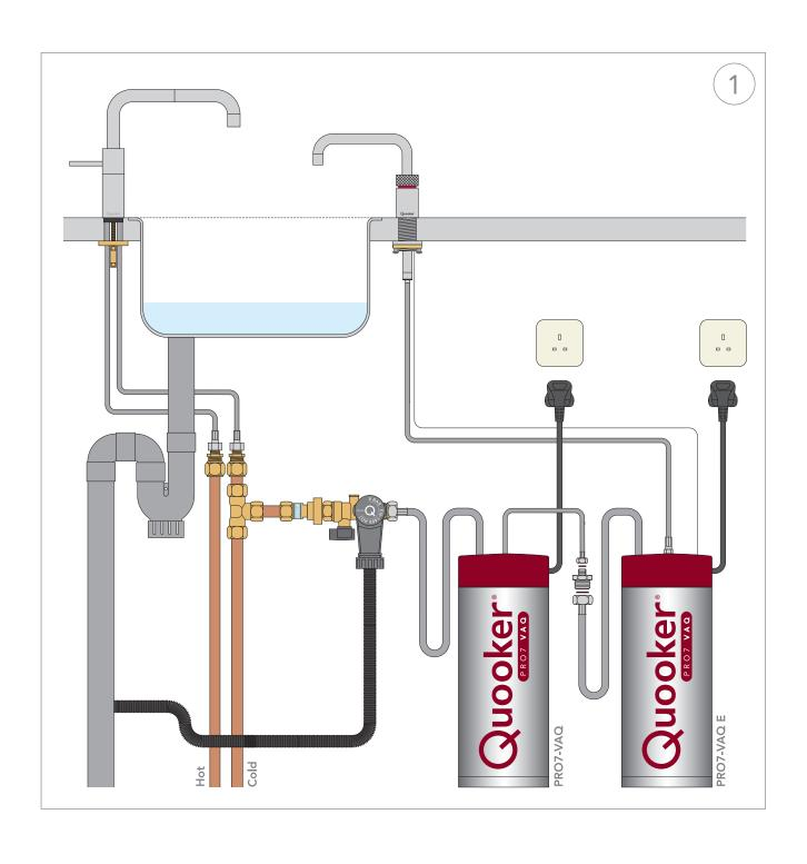
2 The tanks are connected using the included coupling with the accompanying fibre washers.
